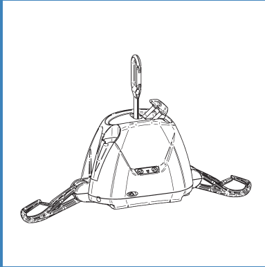
Ceiling Lift - Portable
