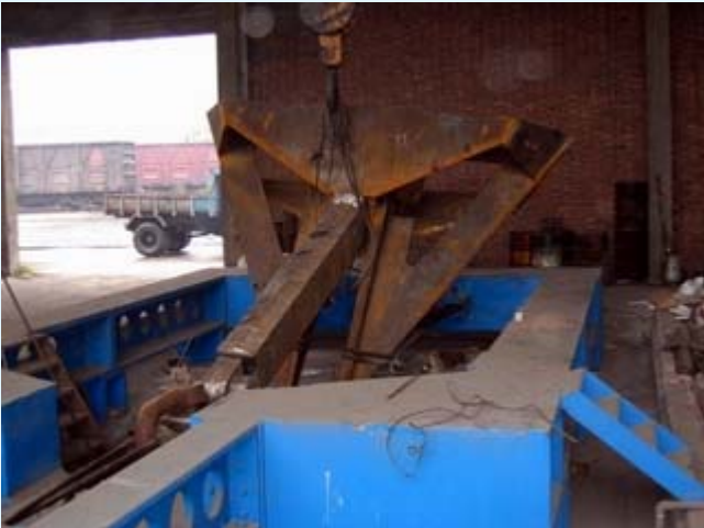
Delta Anchor - Proof Load Test
