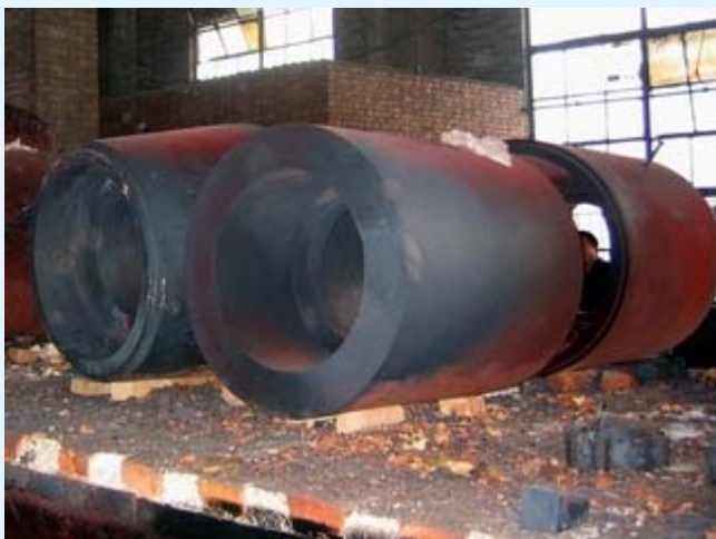
Sterntube - after Heat Treatment
