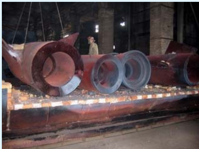
Propeller Shaft Bracket - after Heat Treatment
