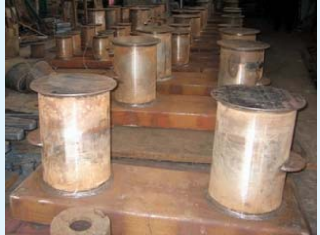
Deck Bollard - Double Bitts
