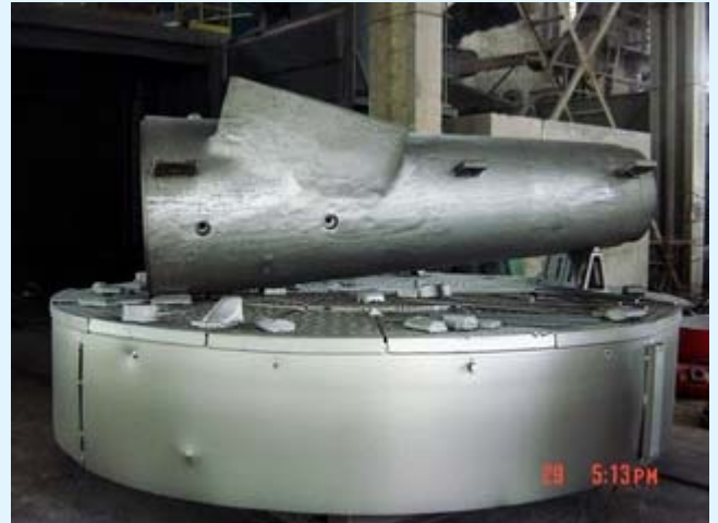
Propeller Shaft Bracket - after Shot Blasting
