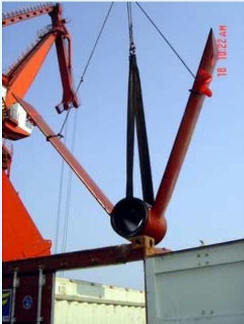
Propeller Shaft Bracket - being Stuffed into Container
