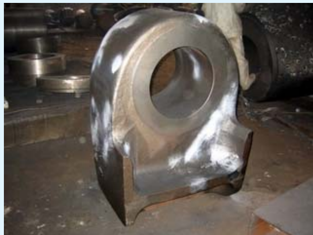
Rudder Carrier - after Magnetic Particle Inspection
