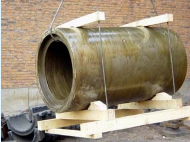
Sterntube - after Application of Anti-rust Oil
