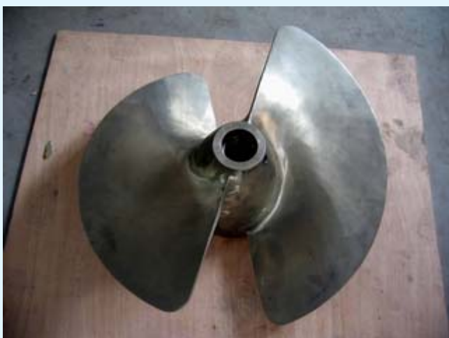
Thruster Propeller - Aluminum
