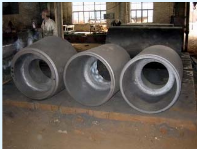
Sterntube - Rough Casting
