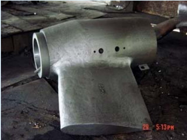
Propeller Shaft Bracket - after Shot Blasting
