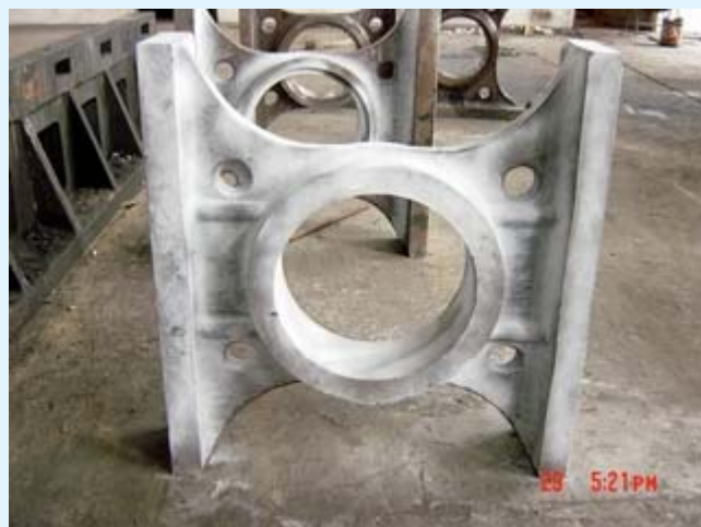
Marine Diesel Engine Crosshead Slipper - after Magnetic Particle Inspection
