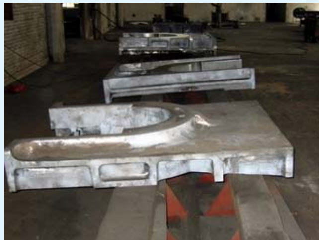
Marine Diesel Engine Main Bearing Support - after Magnetic Particle Inspection
