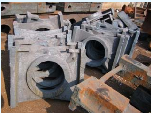
Marine Diesel Engine Crosshead Slipper - Rough Casting
