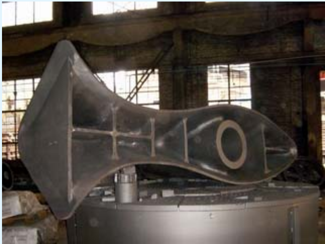
Sternpost - after Shot Blasting
