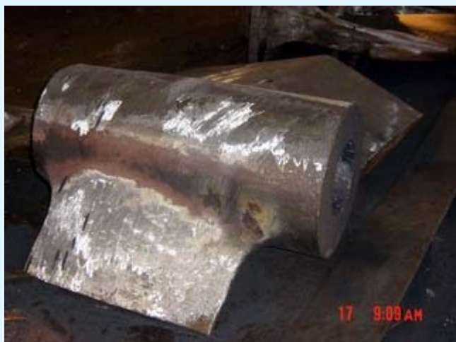
Propeller Shaft Bracket - Rough Casting
