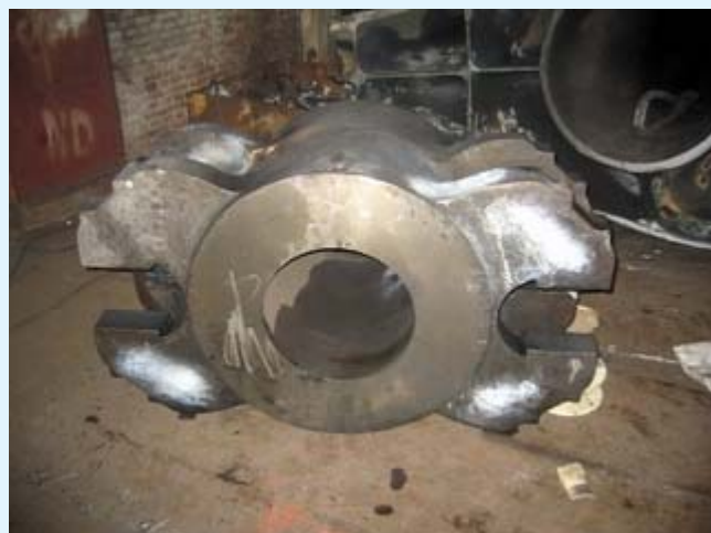
Tiller - after Magnetic Particle Inspection
