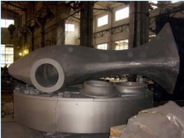
Sternpost - after Shot Blasting
