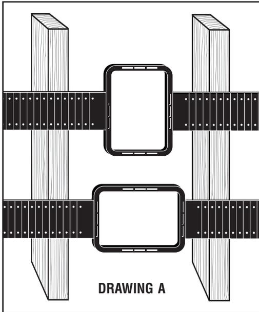
1. Determine the position of your speakers in relation to the wall studs. The Rough-In Kit is designed to accommodate either upright or horizontal mounting positions (examples shown in Drawing A at left).
