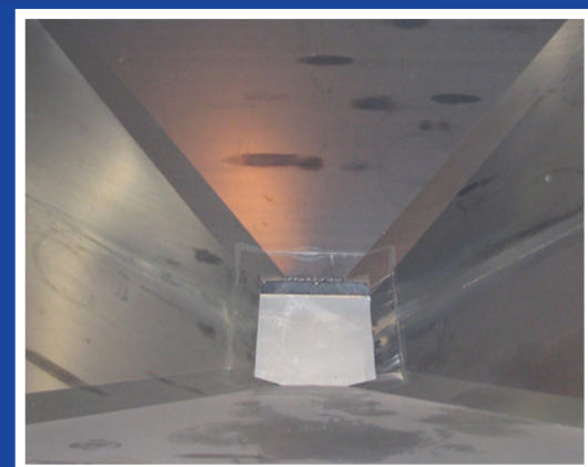
Easy flow hopper with no 90 degree corners to eliminate grain hang-up in corner welds
