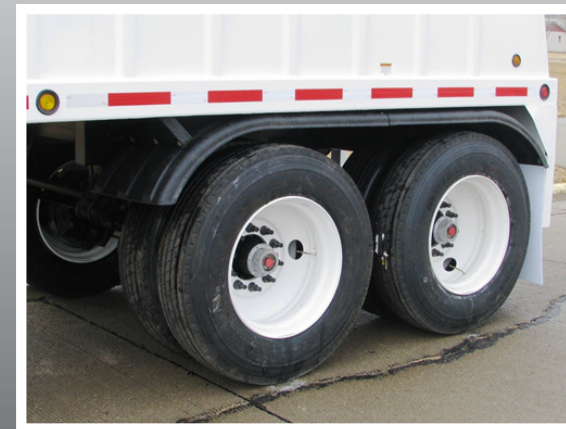
Minimizer fenders to further protect the underside of the trailer from debris
