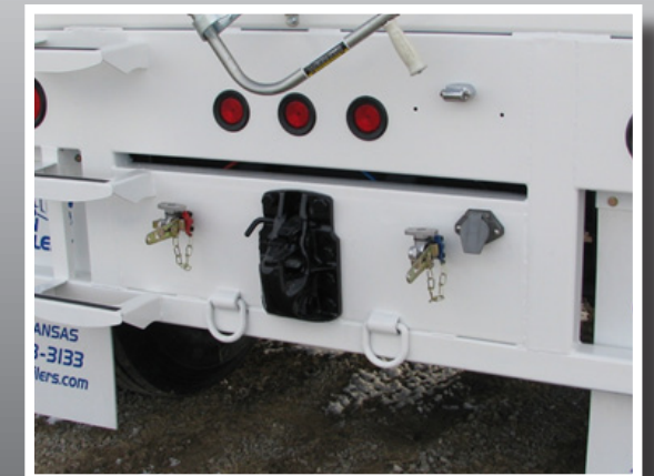
Air-adjusted pintle hook with frame reinforcement, rear gladhands with a built-in shut-off valve and dummy coupling to keep free of debris and 7-way plug
