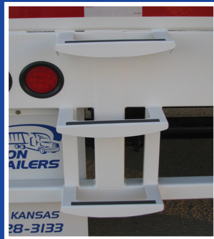
Three additional non-skid steps beneath rear ladder simplify access to the rear of the trailer
