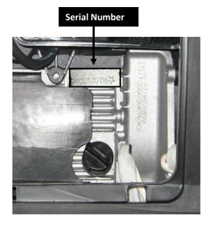
The serial number can be found stamped on the engine block above oil dipstick. It is visible when the maintenance panel is removed.
