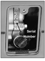
The engine serial number can be found stamped on the engine block above the oil dipstick. It is visible when the engine oil access cover is removed.
