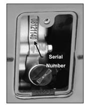
The engine serial number can be found stamped on the engine block near the oil dipstick. It is visible when the maintenance door is removed.
