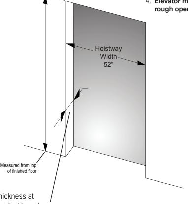
Wall construction and thickness at each landing must be verified in order to determine thickness.
