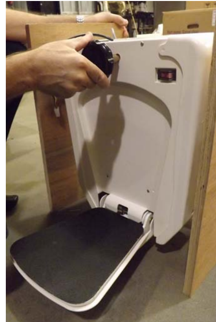
Manual lowering handwheel
