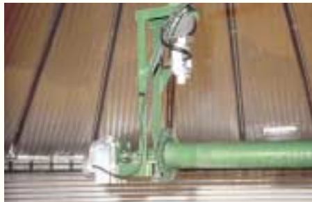
Offset hanger is standard on the Fastir™ to provide more stirring in the center of the bin.
