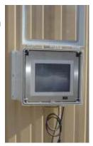
The box that houses the control system weighs less than 15 lbs., so it is easy to handle.
