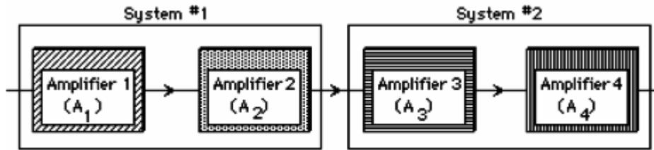
1d: Total Amplification Ratio is invariant under subsystem aggregation—it is associative:
