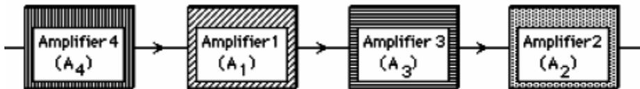
1b: Total Amplification ratio,  $A_t = A_4 \times A_1 \times A_3 \times A_2$  remains unchanged over intersubstitutions changing the order of the amplifiers (or commutation of the A's in the composition function).
