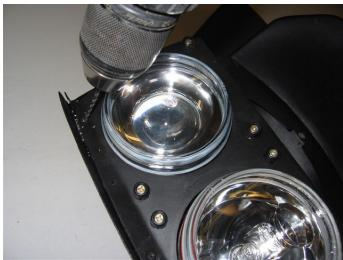
Hold the headlight mount plate in place and carefully drill one of the upper outside holes with a 3/32-drill bit.
