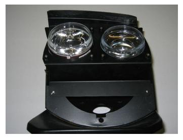
Next put the bezel back on the bulb assembly and test fit the bezel to the bucket once again. The bezel should fit tight and snug with or without the bulbs installed.
