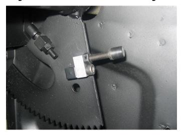
Install the new stop adjuster onto the existing stop adjuster mount like pictured and re-install the original stop bolt.
