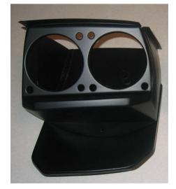
With the center section removed and ground as described, test fit the bezel in each bucket making sure the top and sides are flush with the edges. Late model car may require some grinding on the lower bezel radius to obtain the proper fit.
