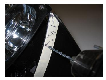
Using a 3/32 bit, dill both sides of the bucket and remove the burrs on the inside left from drilling each hole.
