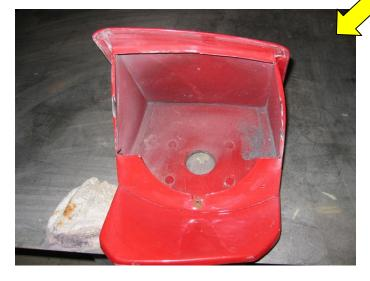
With the center cut out, place the bucket on its side again and start grinding the sheet metal edge down until it is smooth with the inside thickness of the bucket.
