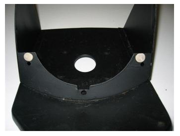
Place a small amount of clay or two-sided tape on the lower corners of light mount plate. This is to help keep the bulbs from moving after they are placed in the bucket while you drill the mount holes and install the screws.
