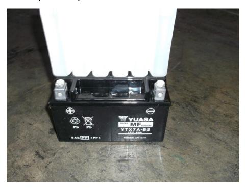
STEP 10.2: ONCE ALL OF THE ACID HAS STOPPED BUBBLING INSTALL THE BATTERY COVER
