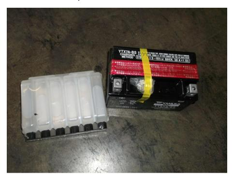
STEP 10.1: PRESS ACID PACK ONTO THE BATTERY AND ALLOW THE ACID TO FLOW INTO THE BATTERY (DO NOT SQUEEZE OR PUNCTURE ACID PACK TO TRY AND MAKE IT FLOW FAST)
