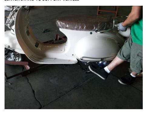
STEP 8: LIFT AND SWING FRONT OF SCOOTER OFF OF METAL FRAME (YOU MAY NEED THE HELP OF AN ASSISTANT TO DO THESE TWO STEP
