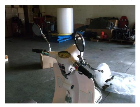
STEP 6: CUT AND REMOVE METAL WIRE TIE DOWNS FROM BOTH SIDES OF VEHICLE
