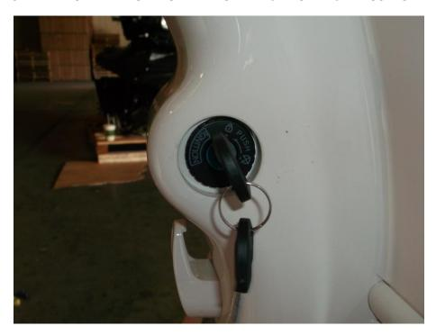
STEP 14.1: PUT THE KILL SWITCH IN THE "RUN" OR "CYCLE" POSITION HOLD THE FRONT BRAKE AND PRESS THE STARTER
