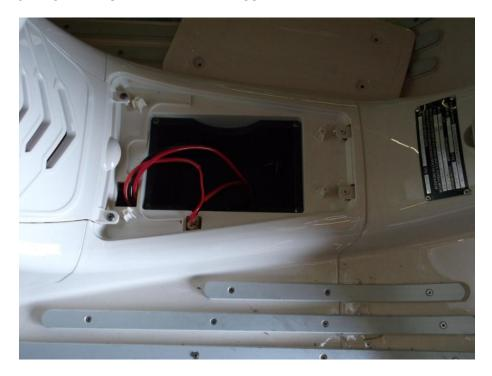
STEP 10: PREP BATTERY FOR ACID BY REMOVING RED FOIL FROM BATTERY, CLEAR PLASTIC FROM ACID PACK AND REMOVE THE BLACK CAP FROM ACID CAP ONLY (DO NOT REMOVE FOIL FROM ACID PACK)
