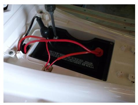
STEP 11.1: INSTALL THE BATTERY COVER WITH 4 SCREWS (USE CAUSTION NOT TO OVERTHIGHTEN THE SCREWS)
