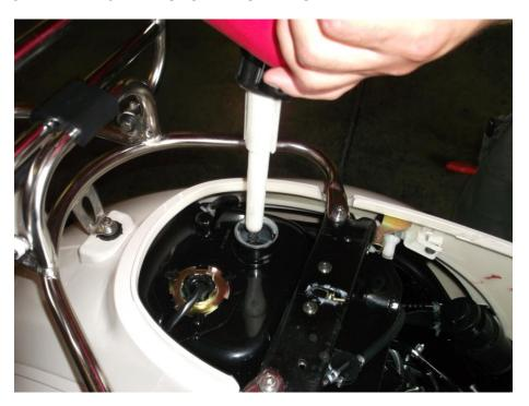
STEP 13: REMOVE THE ENGINE OIL DIP STICK AND VERIFY THAT THE ENGINE OIL IS TO THE FULL MARK ON THE DIP STICK
