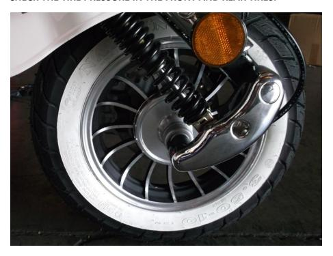
STEP 16.1 CHECK ALL NUTS, BOLTS AND FASTNERS TO INSURE THEY ARE TIGHT (PICTURE SHOWS REAR BRAKE ADJUSTMENT)
