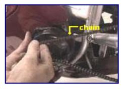
3, Take off the chain and put it aside when the transmission's removed.
