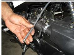
Pull the fuel line until the end is clear of the engine area
