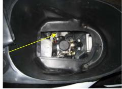
Locate the fuel line leading to the carburetor
