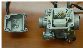
Carb pictured with bowl cover off. Please note that image is of 150cc carb and other carbs may look different
