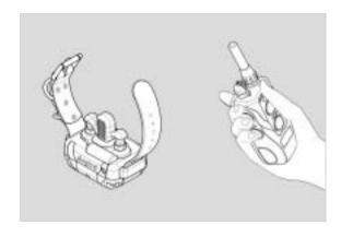
1. To activate the receiver/collar, place the red dot on the back of the transmitter to the red dot on the collar/receiver. Hold the two red dots together for a moment until the LED light on the receiver/collar comes on. The indicator light will come on for a moment then blink once every 4 seconds, showing that the collar is ready to use. (If the indicator light is red, or if there is only 1 bar showing on the battery icon on the LCD transmitter screen, the unit needs to be charged.)
