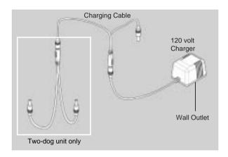
The battery charger and charging cables allow you to charge both the transmitter and receiver at the same time. The battery charger is designed for a 120-volt wall outlet. (European 230-volt AC chargers and 12-volt car chargers for Ni-MH batteries are also available)
