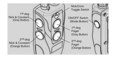
The **dogtra** SUREStim TIDEH two-dog unit has five buttons and a toggle switch on the transmitter. (Two on the face of the transmitter, two on the left side, and one on the right side.)
