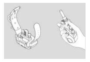
1. To activate the receiver/collar, place the red dot on the back of the transmitter to the red dot on the collar/receiver. Hold the two red dots together for a moment until the LED light on the receiver/collar comes on. The indicator light will come on for a moment then blink once every 4 seconds, showing that the collar is ready to use. (If the indicator light is red, or if there is only 1 bar showing on the battery icon on the LCD transmitter screen, the unit needs to be charged.)
