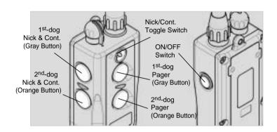
The **dogtrd** 1902NCP Field Star two-dog unit has five buttons and a toggle switch on the transmitter.
