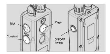
The transmitter for the *dogtrd* 1902NCP Field Star single dog unit has four buttons (one on the face of the transmitter, two on the left side and one on the right side).
