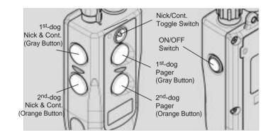
The **dogtrd** 280NCP Platinum two-dog unit has five buttons and a toggle switch on the transmitter.
