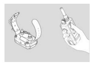
1. To activate your **dogtrd** 280NCP Platinum Series place the red dot on the back of the transmitter to the red dot on the collar/receiver. Hold the two red dots together for a moment until the green colored LED indicator light comes on. The indicator light will blink every two seconds showing the unit is charged and ready to use. (If the indicator light emits a red color, the batteries need to be charged.)
