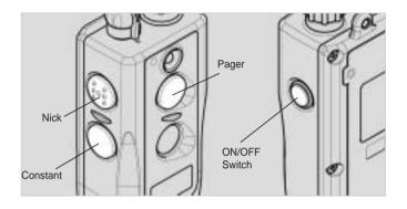
The transmitter for the **dogtrd** 280NCP Platinum single dog unit has four buttons (one on the face of the transmitter, two on the left side and one on the right side).
