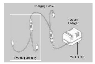
The battery charger and charging cables allow you to charge both the transmitter and receiver at the same time. The battery charger is designed for a 120-volt wall outlet. (European 230-volt AC chargers and 12-volt field charger for your automobile are also available.)
