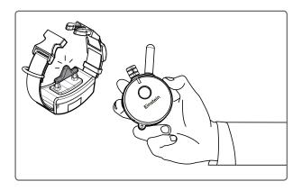
Snap the test light onto the contact points as shown in the above figure. With both units on and green lights flashing, press the continuous stimulation button while turning the stimulation up and down, the test light should brighten as you go higher in stimulation. The collar receiver light will flicker red while the stimulation is on. Next, push the tone button to test the tone feature. Your Einstein E-Collar is ready to use.
