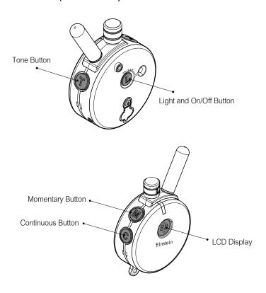
The ET-500 transmitter is equipped with four control buttons, LCD display, and an adjustable dial. For long range use hold the transmitter up like the Statue of Liberty and never allow the antenna to touch anything as it will decrease the range. Power lines and foliage will also reduce the range.
