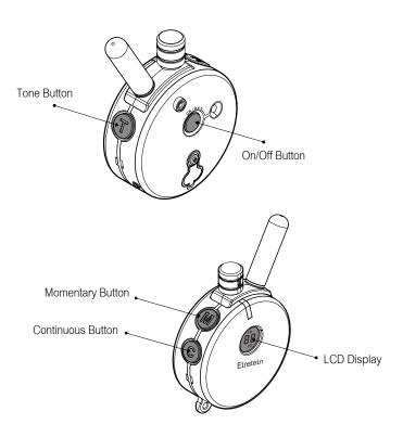
The ET-700 transmitter is equipped with four control buttons, LCD display, and an adjustable dial. For long range use hold the transmitter up like the Statue of Liberty and never allow the antenna to touch anything as it will decrease the range. Power lines and foliage will also reduce the range.
