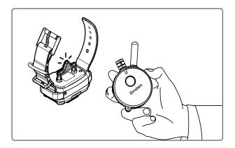
Snap the test light onto the contact points as shown in the above figure. With both units on and green lights flashing press the continuous stimulation button while turning the stimulation up and down, the test should brighten as you go higher in stimulation. The collar receiver light will flicker red while the stimulation is on. Next, push the tone button to test the tone feature. Your Einstein E-Collar is ready to use.
