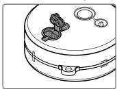
Collar Receiver Battery Charging Receptacle and Rubber Plug
