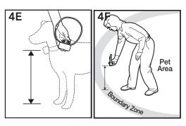
Receiver Collar at your pet's neck level (4F) until the Receiver Collar beeps and the Test Light flashes. If the Receiver Collar beeps before or after the desired Boundary Zone, return to the Transmitter and adjust the Boundary Control Dial. Repeat this process until the Receiver Collar is beeping at the desired location. Record your settings on the next page for future reference.
