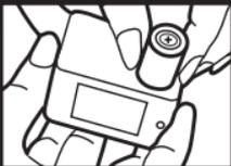
Collar Transmitter: Insert 3v lithium battery in the transmitter positive (+) side out. Replace battery cap.
