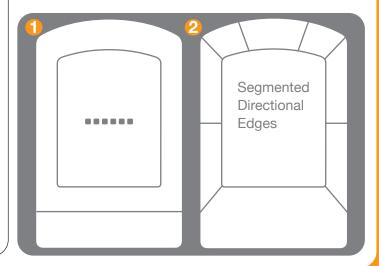
To locate your dog using the Receiver, look at the Display Screen and see which Directional Segment is highlighted. Turn the Receiver until the Directional Segment on the top of the Display Screen begins to strobe; that is the bearing and direction to your dog.
