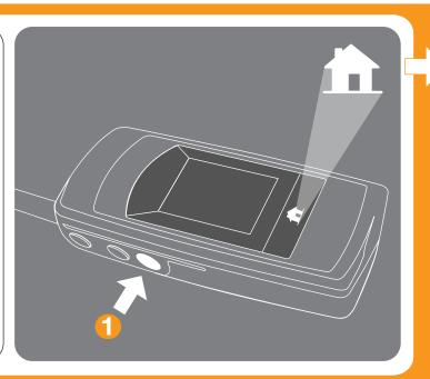
The distance display will show GPS accuracy (e.g. "acc50") and will likely improve over a short time. When the GPS accuracy is down to 15ft or less (e.g. "acc15"), the receiver will now automatically go into Indoor Mode. 1 Toggling the bottom button will turn the Home Mode on and off.
